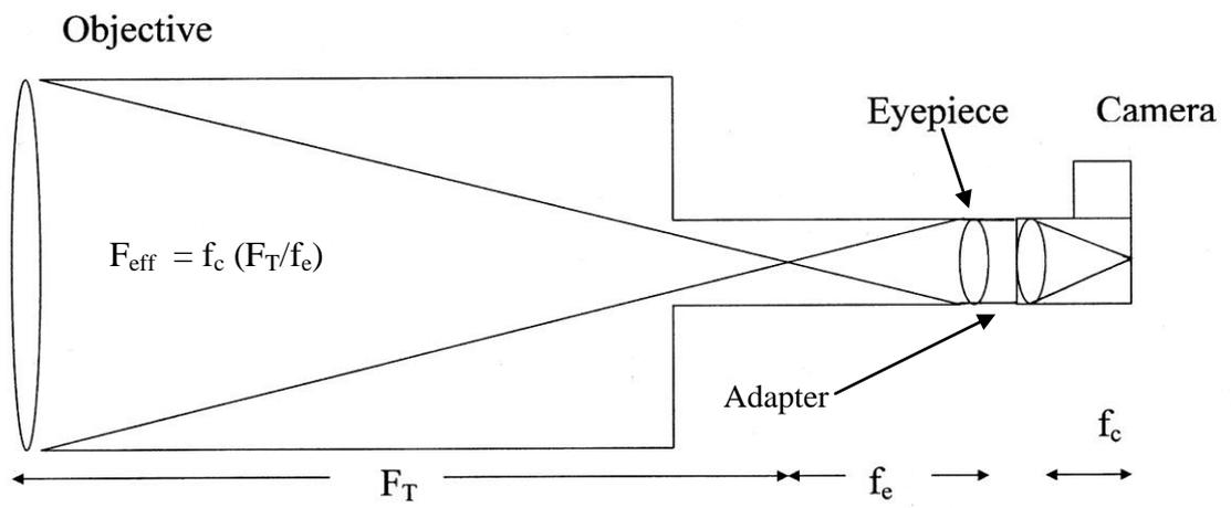
Fig. 4. The afocal method.  $F_T$  = focal length of telescope,  $f_e$  = f. l. of eyepiece,  $f_c$  = f. l. of camera lens,  $F_{\text{eff}}$  = effective f. l.  $F_{\text{eff}} = f_c (F_T/f_e)$
