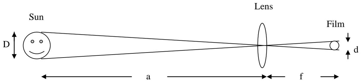
Fig.1.  $D$  is the diameter and  $a$  the distance of the Sun,  $f$  is the focal length of the lens or telescope and  $d$  the diameter of the Sun's image on film.
