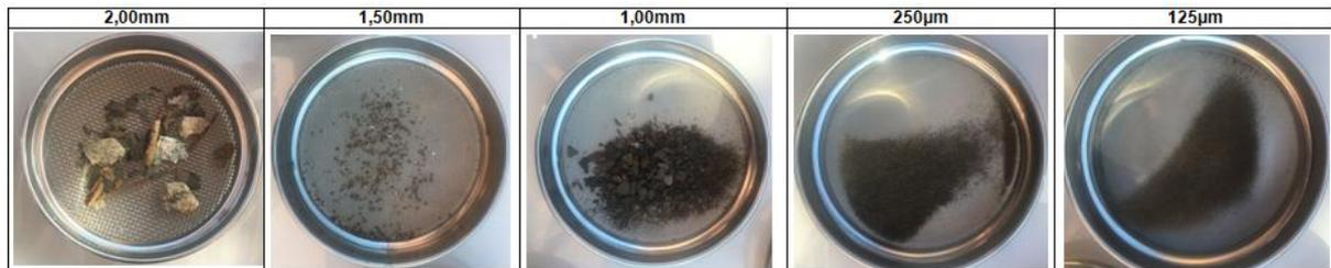
**Image 15.** Classification of metallic waste by size<sup>4</sup> in a single collection.
